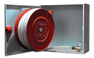
Fire hose cabinet  $\varnothing$ 25 mm according to EN 671-1 standard with 20 m of semi-rigid hose manufactured according to EN 694.
