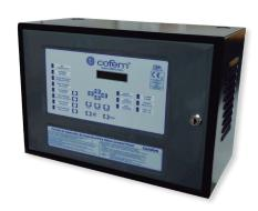
The London control panel allows to connecting up to 10 repeaters, using a 4 wires of 1,5 mm<sup>2</sup> connection (two for supply and two for communication for RS485 line). The two wires of the RS485 line will be connected from the control panel to the corresponding repeaters.
