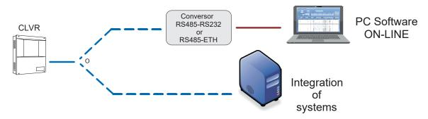
Example of connection for MODBUS functionality
