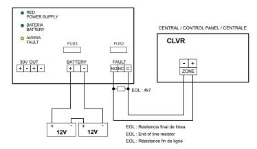
Wiring diagram ZAFIRPWS2/5 fault output
