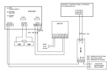
Wiring diagram ZAFIRPWS2/5 Algorithmic Addressable system
