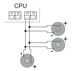
NOTE: Scheme applicable only to zone 3. The other zones are connected in the same way. Control panels with other capacities should not have some connectors.
